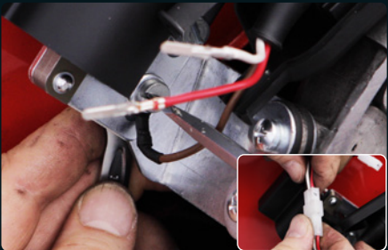
03: Mount coil. Choose suitable holder. Mount and connect plugs. (SIP art.-no. see pages 18 & 19).
