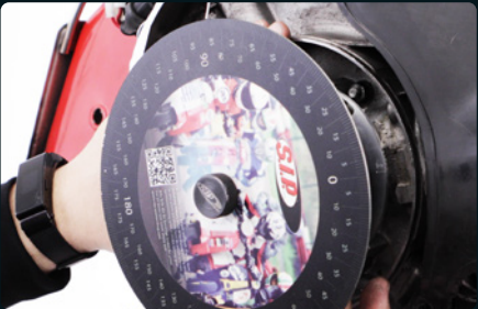
08: Rotate rotor counterclockwise together with locked degree disc against piston stop tool. (Example: 86°)
